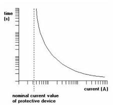
*Fuses operate on the principle of melting when the heat absorbed exceeds its capacity.* Process is usually adiabatic – heat produced goes to heating the fuse wire only.
