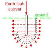
Consider the currents going out from it in a shape of a cylinder and a hemi-sphere at a radius of x as shown.
