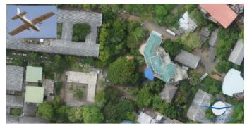
RTK satellite fix. Nevertheless it was possible to reach 4.1cm mean geotagging error with 2.5cm standard deviation. With this accuracy, very precise aerial surveying is possible with the locally developed Drones.
